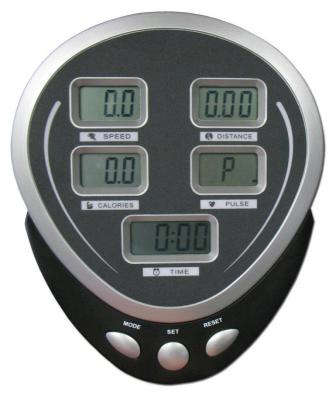
There are 5 seven-segment displays that show program statistics. The four-digit displays are programmed to display time in an 88:88 format.
